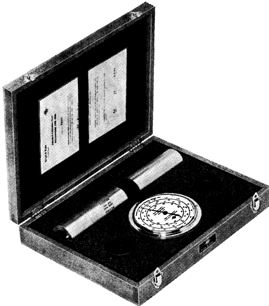
Fig. A.1. The Pistonphone Type 4220 in case with barometer and coupler adaptors for B & K microphones.
